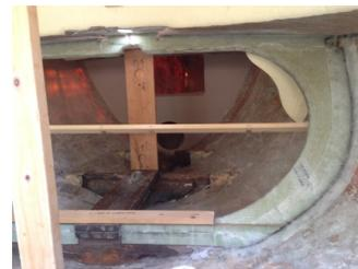
The one piece of decent woodwork was a deck beam and knees assembly immediately forward of the partner. That was made superfluous by a third ring frame, canted to reach from the mast partner across the chainplates to the foremost set of keel bolts. It too is made of foam core board, so weighs only 7 lb. 4 oz.
